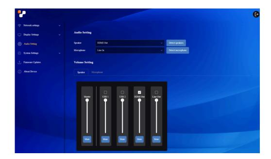
Here you can test whether the speakers and microphones that connected to the device are available or not. You can also select which available speaker output and corresponding volume adjustment, and select which available microphone input and corresponding volume adjustment.
