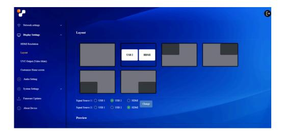
In PBP mode, you can select two signal sources at the same time and then they will be output and displayed on the same screen in the same proportion, one on the left and one on the right. For example, You can directly click Signal Source 1 and Signal Source 2 with the mouse. When the green button of the corresponding interface lights up, this signal input source is output and displayed on the screen.
