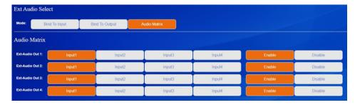
**Audio Matrix**: you can select the audio of any HDMI input source for the corresponding extaudio out.
