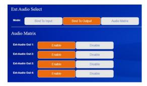
Bind to Output: The AUDIO OUT (1~4) follows the HDMI OUTPUT (1~4). For example, if HDMI INPUT 2 is assigned to HDMI OUTPUT 1, the audio of AUDIO OUT 1 is from HDMI INPUT 2; if HDMI INPUT 3 is assigned to HDMI OUTPUT1, the audio of AUDIO OUT 1 is from HDMI INPUT 3. The audio out channel can be enabled or disabled if needed.
