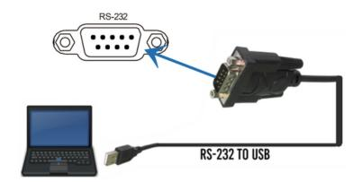
Then, open a Serial Command tool on PC to send ASCII command to control the Matrix. The ASCII command list about the product is shown as below.
