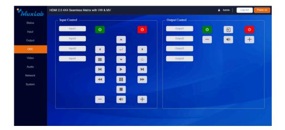
You can perform CEC management on this page. Inputs and Output scan be controlled by clicking on the corresponding icons.
