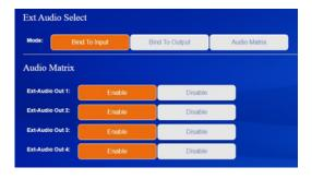
**Bind to Input**: The AUDIO OUT  $(1\sim4)$  follows the HDMI INPUT  $(1\sim4)$ . And there is a consistent one-to-one match between each HDMI input and audio output.
