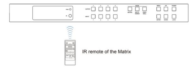
The second way: If the IR receiver window of the Matrix is blocked or the Matrix is installed in a closed area out of infrared line of sight, the IR receiver cable can be inserted to the "IR EXT" port to receive the IR remote signal. The furthest distance of using the IR remote is 5 meters when the IR remote is directly faced to the IR receiver head, and 3 meters when the using angle is  $\pm$  45°. The diagram is shown as below.
