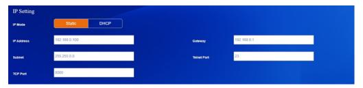
If the Mode is "Static", you can set manually the IP Address/Gateway/Subnet/Telnet Port as required.
