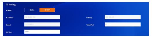
If the Mode is "DHCP", it will search and be filled with the IP Address assigned by the router automatically. You can't modify it now.
