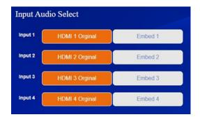
You can select any input audio source from an HDMI input internal audio or an embedded audio. For example, if "HDMI 1 Original" is selected, the audio source is from the internal audio of HDMI Input1; if "Embed 1" is selected, the audio source is from the Embed 1 audio. (The embed audio follows HDMI INPUT, and it will be embedded in HDMI INPUT to output.) The ext-audio has three modes: Bind to Input, Bind to Output and Audio Matrix.
