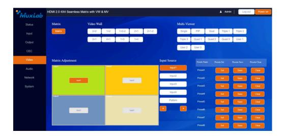
In matrix mode, you can selectan output  $(1\sim4)$  firstly, and then selectan input source  $(1\sim4)$  which will appear on the selected output area. One route of video output configuration is completed.
