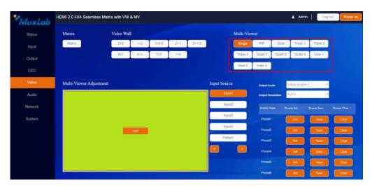
In multi-viewer mode, all the four HDMI outputs display the same image from the HDMI IN you selected. You can select the input source which will appear on the corresponding window area. Then set the output resolution for current output by clicking the drop- down list. Output Audio can be selected to follow any input source or the corresponding window as required.
