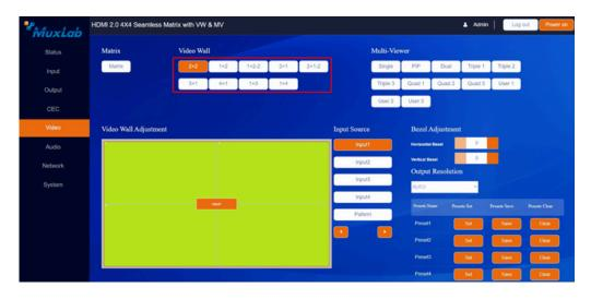
In video wall mode, you can select a window  $(1\sim4)$  firstly, and then select an input source  $(1\sim4)$  which will appear on the selected output area. Click+/- to adjust the corresponding Horizontal/Vertical Bezel (0-10). Set the output resolution for current output by clicking the drop-down list.
