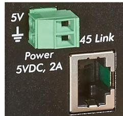
**Note: Power the HDMI Wall-Plate Extender Balun only after all connections are made.**
