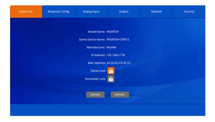
In this page, it shows the model name, device name, IP address and MAC address.
