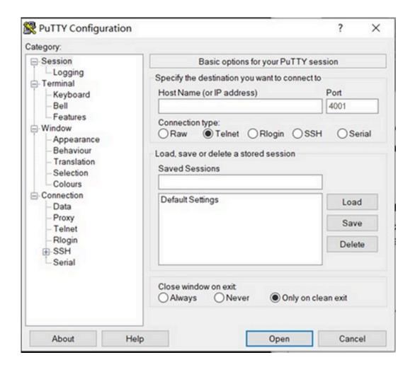
Firstly, type in the IP address of GUI in "Host Name" and the port is 4001, chose Telnet connection type, then click the open, and a new window will pop up. Then the user can send commands to control the Dante device.
