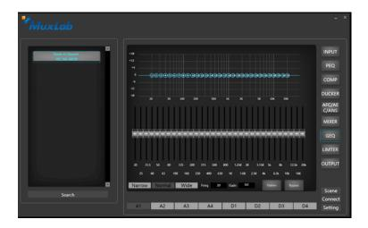
The gain of 31 frequency points can be adjusted individually, to achieve the purpose of strengthening or weakening certain frequency points and achieve different effects.
