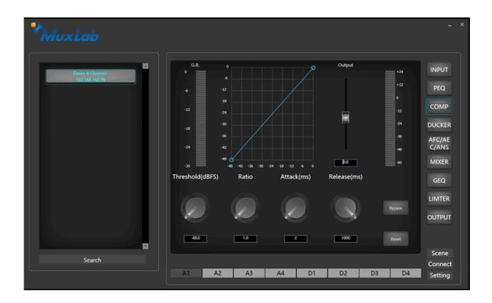
**Threshold**: Threshold value of the compressor.
