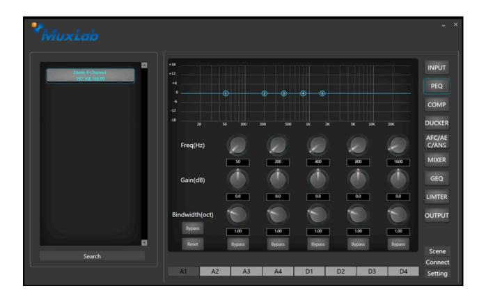
**Equalizer type**: 5-terminal parametric equalizer
