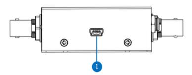
1. Mini-USB connector to connect a PC running the MuxLab SDI Manager Software.
