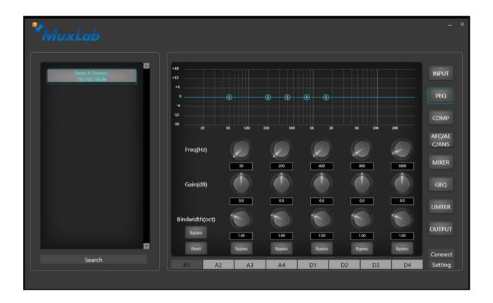
**Equalizer type**: 5-terminal parametric equalizer
