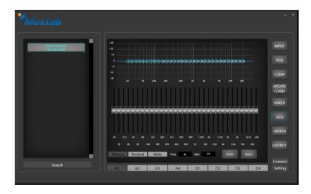
The gain of 31 frequency points can be adjusted individually, to achieve the purpose of strengthening or weakening certain frequency points and achieve different effects.
