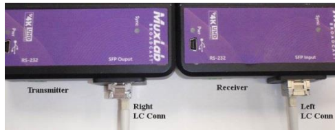
Figure 6 Connecting the Fiber Cable
