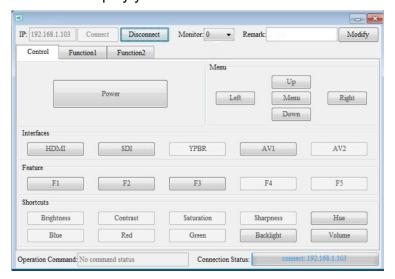
If the unit is connected, the IP will be displayed at the bottom
