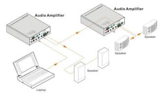
Figure 4-3 Cascade Connection
