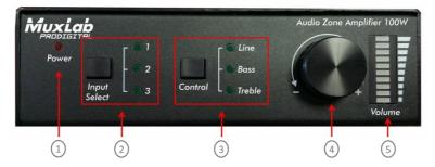
Figure 2-1 Front Panel of Zone Audio Amplifier
