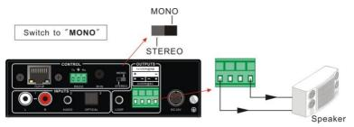
Figure 4-2 Mono Output Connection
