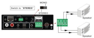
Figure 4-1 Stereo Output Connection
