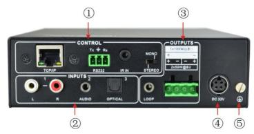
Figure 2-2 Rear Panel of Zone Audio Amplifier
