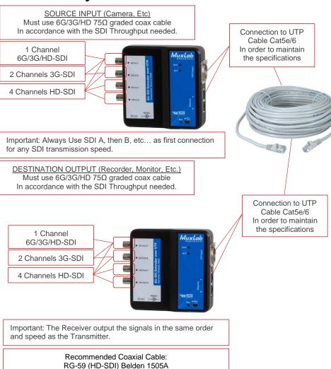
Figure 4: Physical Installation
