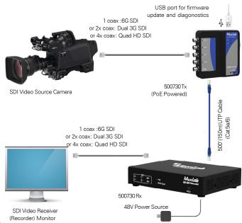
Muxlab's CAT 5/6 cable transfers 4K video to a distance of 150 meters
