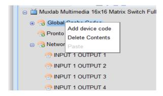
3) A new device code will appear at both the bottom-left and upper-right corners of the screen. Update the name field as desired and paste the RS-232 data taken from the "Network codes" section.
