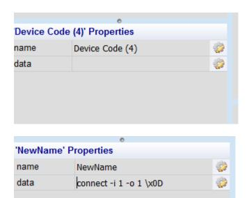
4) To make use of this new command on your project interface, drag and drop the new RS232 command (action) on top of a newly created button within your project interface. Once done
