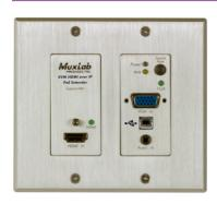
The HDMI/VGA/USB over IP PoE Wall Plate Transmitter allows HDMI, VGA and USB equipment to be connected up to 330ft (100m), with video supported at up to 4K (3840x2160) resolution @ 30Hz via one CAT5e/6 unshielded twisted pair cable in a point-to-point configuration. Point-to-multipoint and multipoint-to-multipoint configurations are also possible by connecting several Transmitters and Receivers to the same local Ethernet IP network via an Ethernet Switch.
