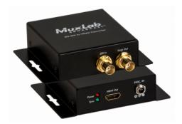
The 3G-SDI to HDMI Converter allows SDI equipment to be connected to an HDMI Display. The unit converts the SDI signal to HDMI, supporting resolutions of 480i (SD-SDI), 720p/1080i (HD-SDI) and 1080p (3G-SDI). The 3G-SDI to HDMI Converter provides a low jitter and re-clocked outputs allowing for unit daisy chain.
