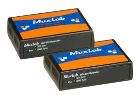
The 3G-SDI Extender allows 3G-SDI to be transmitted up to 330ft (100m) via Cat5e/6 cable in a point-topoint configuration. The 3G-SDI Extender supports transmission of up to 2.97/3.0Gbps uncompressed, un-encrypted digital video (optionally including embedded Audio and/or Time Code) within television facilities and between professional video equipment.
