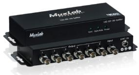
The 12G-SDI 1x6 Splitter, 4K/60 allows one (1) 12G/6G/3G/HD/SD-SDI source to be distributed and amplified to up to six (6) 12G/6G/3G/HD/SD-SDI displays. The splitter supports up to 4K (3840 X 2160) video and HD audio, including 480i (SD-SDI), 720p/1080i (HDSDI), 1080p (3G-SDI), 4K/30 (6G-SDI) and 4K/60 (12G-SDI).
