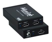
The DisplayPort 1.2a 1x2 Hub, MST (500506) is a device that allows you to extend different DisplayPort 1.2a content from one DisplayPort connector to two monitors. The hub supports video resolutions up to 4K and PCM Audio up to 7.1-Channel and up to 192 kHz sampling rate, and supports Multi-Stream Transport (MST) of up to eight streams.
