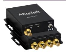
The 3G-SDI 1x4 Splitter allows one (1) 3G/HD/ SD-SDI source to be distributed and amplified to up to four (4) 3G/HD/SD-SDI displays. The splitter supports up to 1080p video, including 480i (SD-SDI), 720p/1080i (HD-SDI), and 1080p (3G-SDI). The device automatically detects the 3G/HD/SD-SDI signal and re-clocks and regenerates the signal at the output for extending distances between source and displays.
