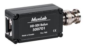
The HD-SDI Balun allows one HD-SDI signal to be transmitted up to 150ft (45m) via Cat5e/6 cable at HD resolution in a point-to-point configuration. The HD-SDI Balun supports transmission of up to 1.5Gbps uncompressed, un-encrypted digital video (optionally including embedded Audio and/or Time Code) within television facilities and between professional video equipment.
