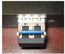
3c. Connect one single-mode optical fiber cable to the left side of the LC connector on the Transmitter. Retain the plug and replace it on the LC connector if the fiber cable is not present. Note that the right side of the LC connector is not used on the Transmitter. If only one optical cable is used, plug the unused LC connector.
