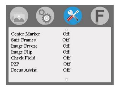
Center Marker: Use to set the center mark (cross mark) on the display.
