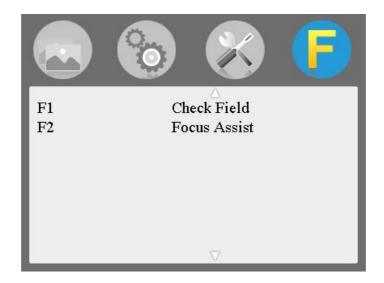
F1: Setting custom button F1: Select custom button "F1", press the ">" or "<" button to pop-up the "F" button functions and select between (Center Marker, Safe Frames, Check Field, Focus Assist, Aspect Ratio, Image Flip, Pixel to Pixel "P2P", or Image Freeze). Then press the "^/F1" button to assign it to the "F1" custom button, then press the "MENU" button to confirm.
