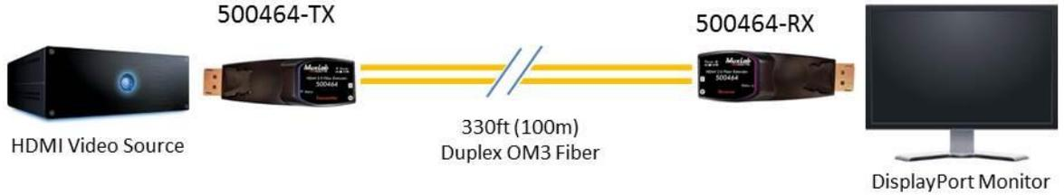
Up to 4K Resolution @ 60Hz over 100m of OM3 Multi-mode Fiber
