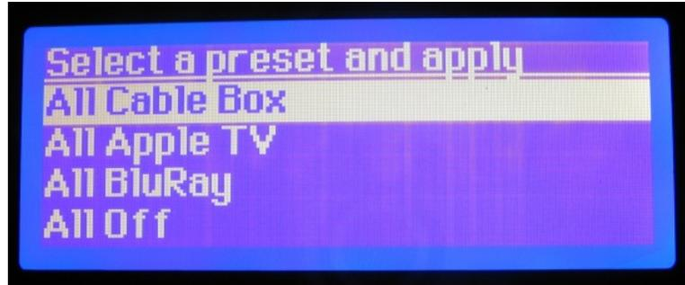
Once selected, the user presses the Enter/Save button on the numeric keypad. The Select a Preset and Apply screen then confirms the selection.
