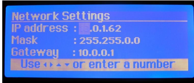
The user navigates the Network Settings screen using the arrow keys, and enters information using the numeric keypad.
