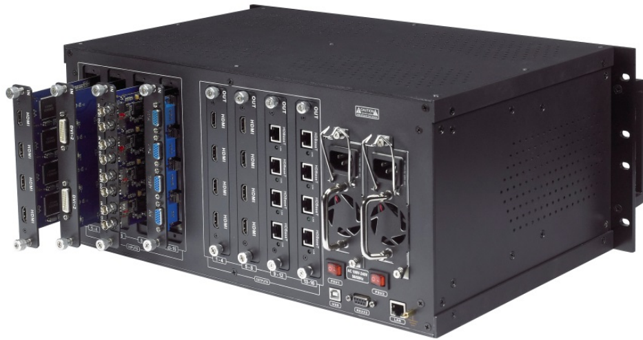
Figure 7: Back Panel with Removable Card Modules
