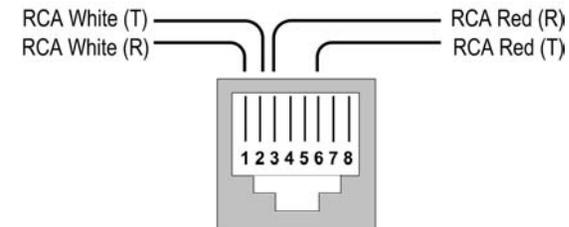
**Note:** The Stereo Hi-Fi Balun is phase polarity sensitive. Therefore, in order to achieve full stereo audio quality, please ensure that the wiring is straight-through and according to EIA568 (A or B) standard.
