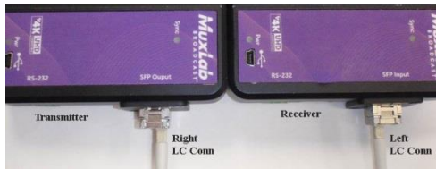
Figure 6 Connecting the Fiber Cable
