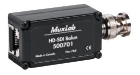
The HD-SDI Balun allows one HD-SDI signal to be transmitted up to 150ft (45m) via Cat5e/6 cable at HD resolution in a point-to-point configuration. The HD-SDI Balun supports transmission of up to 1.5Gbps uncompressed, un-encrypted digital video (optionally including embedded Audio and/or Time Code) within television facilities and between professional video equipment.
