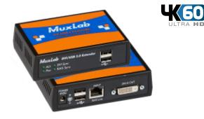
The DVI / USB2.0 HDBaseT Extender Kit (500391) allows one DVI channel and one USB2.0 channel to be transmitted up to 330ft (100m) at all resolutions up to 1920x1200 via single Cat5e/6 cable, and up to 230ft (70m) at 4K (3840x2160). The Receiver features a 4-port USB2.0 hub for transferring multiple USB2.0 data transmissions, well suited for KVM applications.
