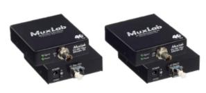
The 6G-SDI Fiber Extender Kit allows 6G-SDI to be transmitted up to 60,000ft (20km) via a one singlemode fiber cable in a point-to-point configuration at all specified bit rates. The 6G-SDI Fiber Extender Kit supports transmission of up to 6.0Gbps of digital video within television broadcasting facilities and between professional video equipment.
