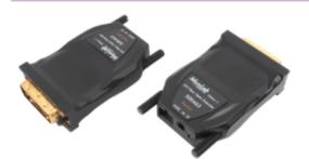
Extend DVI over one multimode fiber optic cable up to 3,280ft (1km). The MuxLab DVI Fiber Optic Extender Kit lengthens your DVI display from your video source using a single strand of multimode fiber optic cable. Automatic EDID programming enables simple synchronization of the video source to the display.
