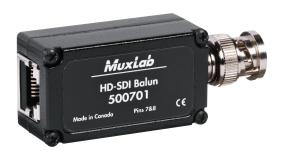
The HD-SDI Balun allows one HD-SDI signal to be transmitted up to 150 ft (45m) via Cat5e cable at HD resolution in a point-to-point configuration. The HD-SDI Balun supports transmission of up to 2.97/3.0 Gbps uncompressed, un-encrypted digital video (optionally including embedded Audio and/or Time Code) within television facilities and between professional video equipment.
