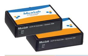
The CCTV IP Extender Kit (500110) allows any CCTV IP camera to be connected over extended distance via Cat5e or coax cable. The 500110 supports up to two IP cameras up to 650 ft (200m) at 100 Mbps and up to 1 mile (1.6km) at 25Mbps.
