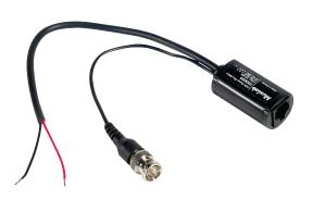
The CCTV Power-Thru Balun allows video and remote power to be transmitted via one 4-pair Cat5e/6 cable, thus eliminating the need to install multiple cables for more efficient cabling in the CCTV security and surveillance environment. The Power-Thru Balun may be used in pairs or in conjunction with standard twisted pair crossconnect devices and other MuxLab CCTV baluns such as the 500000, 500009, 5000023 and 500015.
