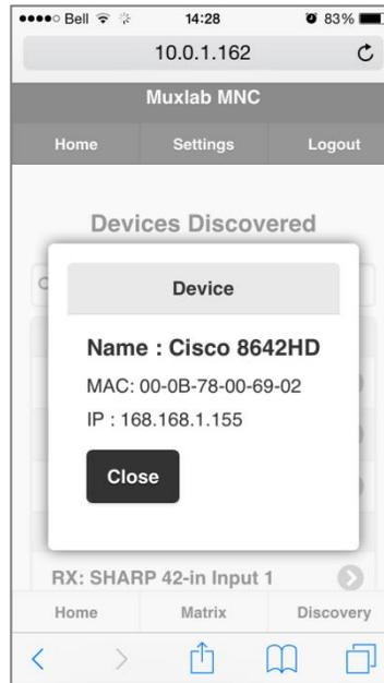
After selecting any Source or Display from the list, the user is presented with the MAC and IP Address of the device in question.
