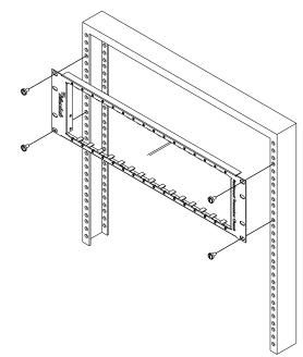
Attach two brackets on the sides of each transceiver. Brackets can use the same screws used on the transceivers. Simply remove the screws on one side of the transceiver, place one bracket and put back the 2 screws. Attach the second bracket in the same way.
