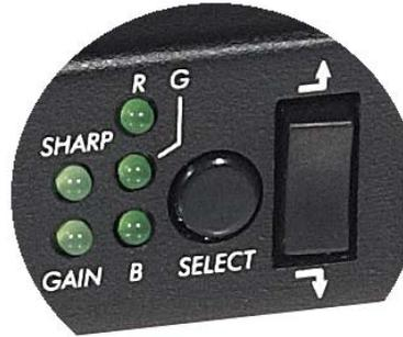
**Figure 8: Manual Image Control Buttons and LEDs**
