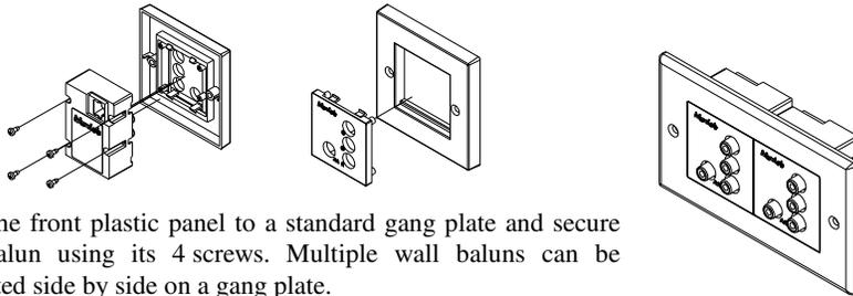
9. Clip the front plastic panel to a standard gang plate and secure the balun using its 4 screws. Multiple wall baluns can be mounted side by side on a gang plate.
