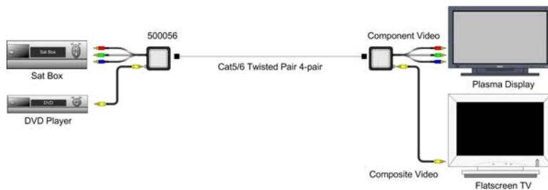
6. Power-on the component video equipment. Check the image quality and refer to the troubleshooting table below if the image quality is unsatisfactory. The following diagram shows a typical installation.
