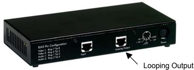
For example an audio video presentation from a VCR or DVD source may be distributed to multiple classrooms via pre-installed Cat 5 twisted pair cable. Due to the active electronics in the hub, the number of hubs that may be cascaded is eight (8).
