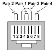
Assuming the spare pairs are available, the two spare twisted pairs could be diverted to a second and/or third RJ45 outlet at both ends. This would allow up to two audio-video channels to be transmitted via Cat5 between the two locations. The following diagram shows how the two spare twisted pairs could be used to transmit stereo-audio or composite video and monaural audio from one room to another.
