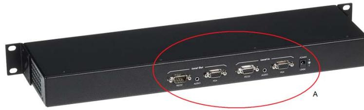
Figure 3: Back Panel of Dispatcher
